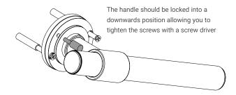
Rear-view of lever showing install pin in postion.
