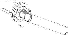
Rear-view of lever showing install pin in postion.
