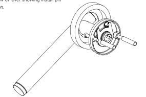
Once secured, reinstall rosette covers by hand and remove plastic covering
