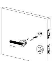
6. Loosen rosette cover from lever and install 2x M4x15 screw to the Lever
